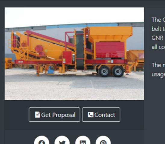
The GNR ME1650 Mobile Screening Plant can be fed with loaders in sand or mines, or connected by a belt to another crushing screening plant in use.
